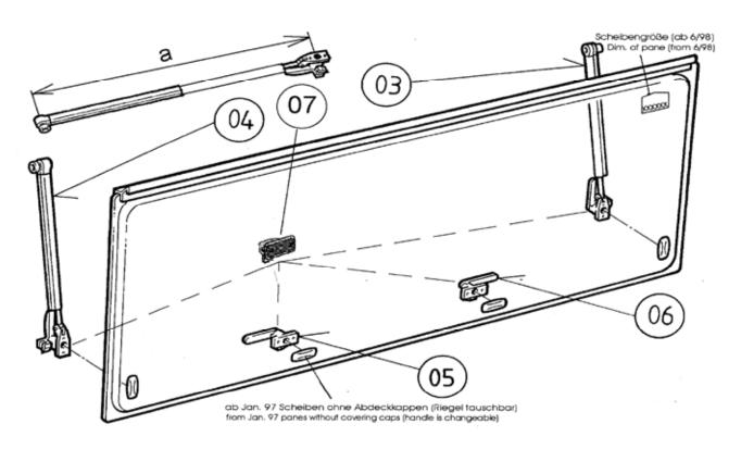
ALL SEITZ WINDOWS CARRY A SMALL IDENTIFICATION TAG ON THE GLAZING PANEL THIS SHOULD CONTAIN THE MEASUREMENTS OF THE WINDOW AND THE STYLE FOR EXAMPLE AGS51000X0600 AN S5 WINDOW MEASURING 1000mm BY 600mm YOU WILL NEED THIS TO COMPLETE PART NUMBERS CONTAINING (\*\*\*\*X\*\*\*\*)
