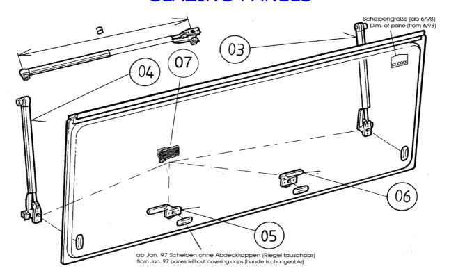
ALL SEITZ WINDOWS CARRY A SMALL IDENTIFIACTION TAG ON THE GLAZING PANEL THIS SHOULD CONTAIN THE MEASUREMENTS OF THE WINDOW AND THE STYLE FOR EXAMPLE AGS41000X0600 AN S4 WINDOW MEASURING 1000mm BY 600mm YOU WILL NEED THIS TO COMPLETE PART NUMBERS CPNTAINING ((x code)X(y code))
